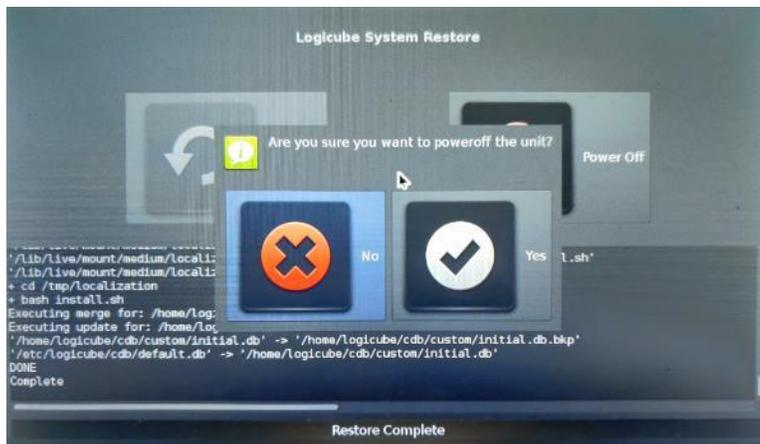
13. The Falcon-NEO should gracefully shut down and will turn itself off. The System Restore process should now be complete. Disconnect the USB keyboard and turn the Falcon-NEO on to make sure it boots properly.
