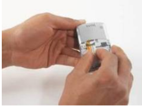
Removing SIM card from cell phone
